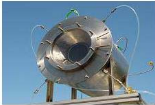
Fig. 1: Front view of the solar water-splitting receiver-reactor [1]
