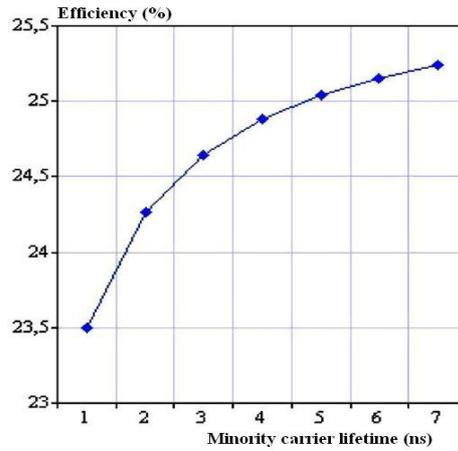
Fig. 1: Effect of minority carriers lifetimes on the conversion efficiency of a single junction  $In_{0.53}Ga_{0.47}N$  solar cell.
