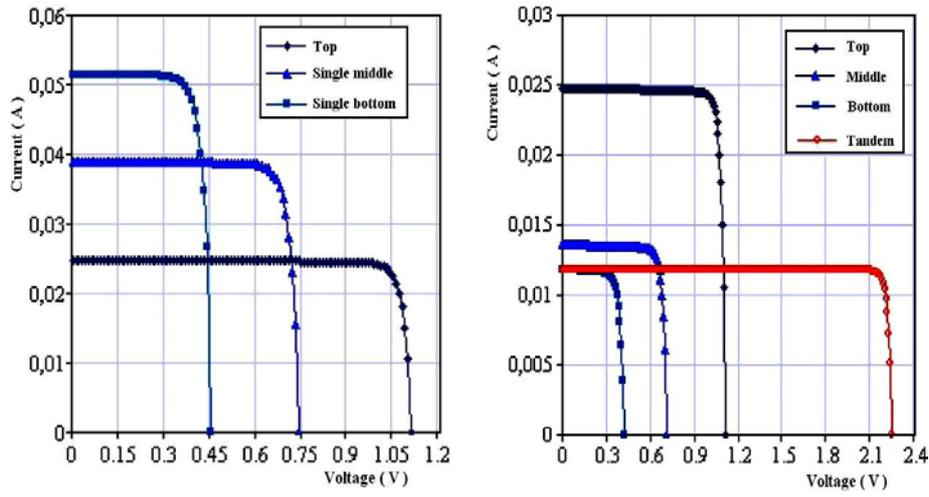
Fig. 4: Simulated I (V) characteristics of the triple junction tandem: (left) for top, middle and bottom single junctions, (right) for top, middle, bottom and the tandem
