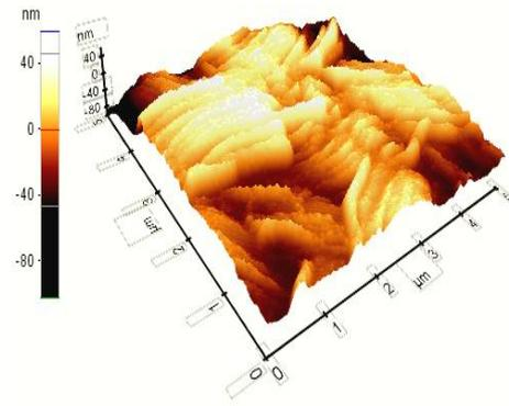
Figure 4. 3D-AFM view of spin coated ZnO film.
