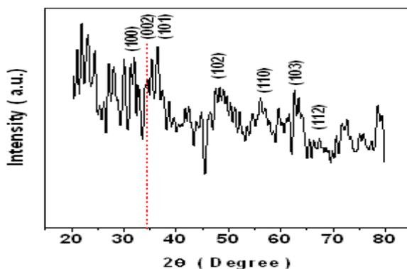
Figure 1: X-rays pattern of zinc oxide at room temperature; two-theta range is  $20^\circ$ - $80^\circ$ . Red dash line locates the peak (002) at  $34.42^\circ$ .
