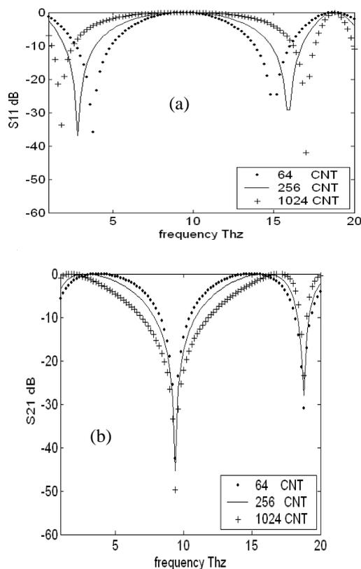
Fig-4 Scattering parameters with variant number of nanotubes
